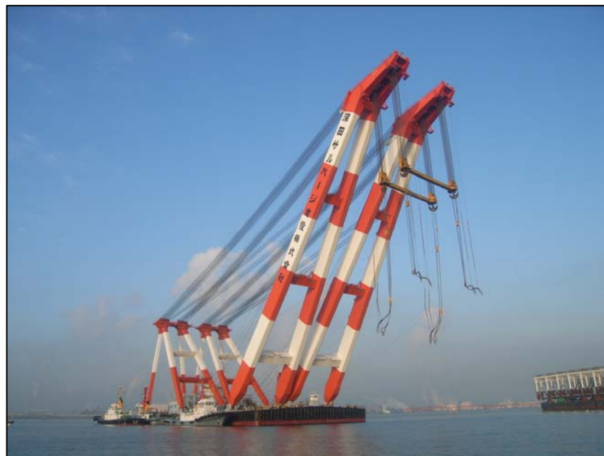
3,700t 吊起重機船 (武蔵)
